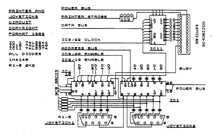
maximum length of the printer cable is 2 meters. Any greater and a problem known as 'skew' arises. Skew is where data bits arrive at the printer at different times. Some simple tests on my interface shows that the full alphabet can be sent to the printer in about 10 milleseconds (1/100 sec). This equates to a transfer rate of about 2,600 characters per second. The fact that most printers print 150 characters or less per second proves the need for the BUSY line.
